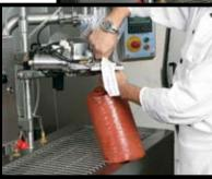
Station-mounted clipper for sealing, attaching label and trimming casing
